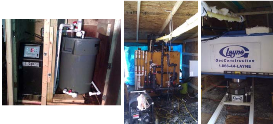
Thermo-mechanical Load Test Set-up
